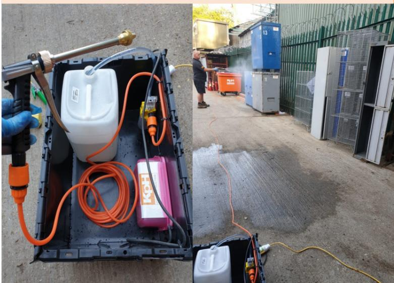
In response to the industry wide shortage of RPE, KPH have responded through innovation. Whilst Dust Suppression systems are nothing new, they can be costly. We looked at various ways we could improve on the current hand pump systems and our logistics co-ordinator Alex Terinte came up with this idea. It allows us to spray a fine mist powered via site temporaries, over a wider area and is portable. This is a perfect solution when working on refurbishment projects avoiding the risk of saturation.
